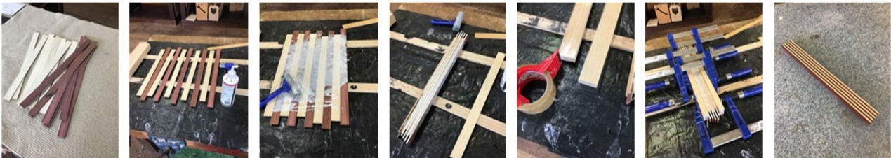
Images TG1-TG7: Example of LVL style material glue-up
