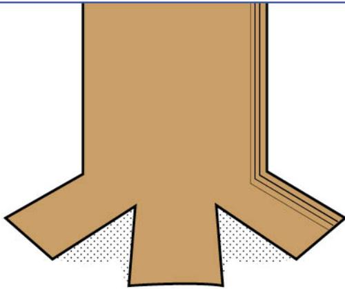
Cut the end of a tube into a fan to attach it to a flat object.
