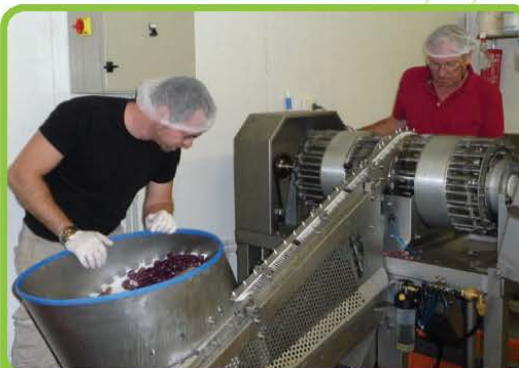
Jose Gomez Luna (left) from Seville in Spain and Eric Dixon experiment with WA's first pitting and slicing machine. Customers were craving local fresh pitted olives and the Bunters and Dixons took the opportunity to do the market research, purchase the technology, and deliver.
